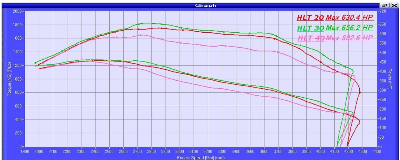
This dyno graph shows the result of over advancing the timing.
